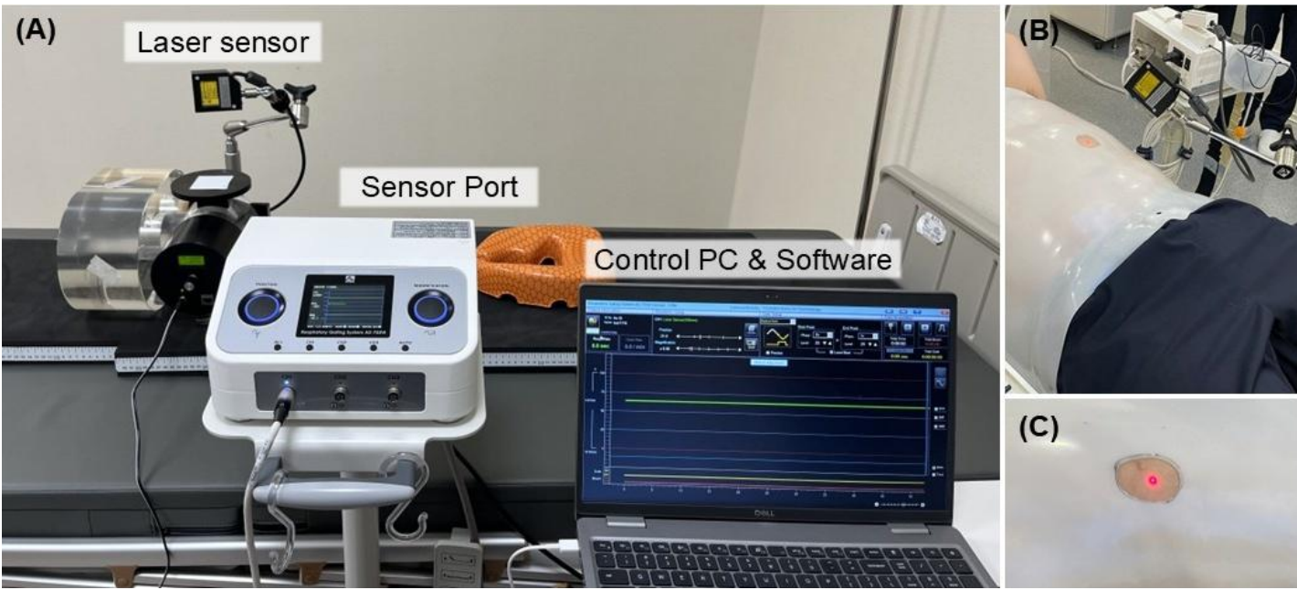
Figure 1. ANZAI laser-based respiratory gating system and clinical setup using a thermoplastic immobilization shell. (a) System configuration showing the laser sensor, sensor port, control personal computer (PC), and software interface. (b) Clinical setup of the laser sensor positioned above the shell for respiratory motion tracking. (c) Opening in the shell enabling unobstructed laser projection onto the patient's skin for accurate signal acquisition.
